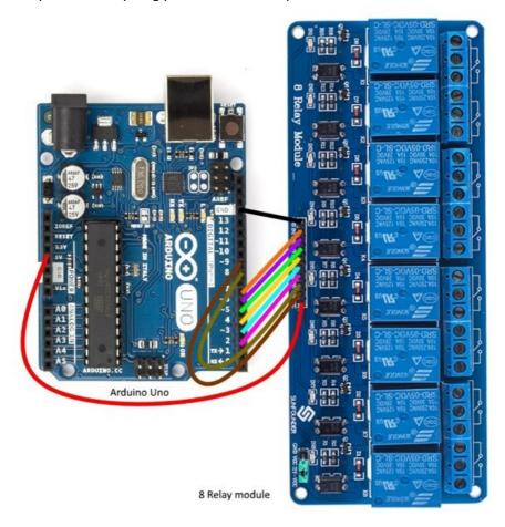
In this picture on the Arduino is wired from pin 9 to pin 2. Don't it will not work wire it up from pin 12 to pin 5.
